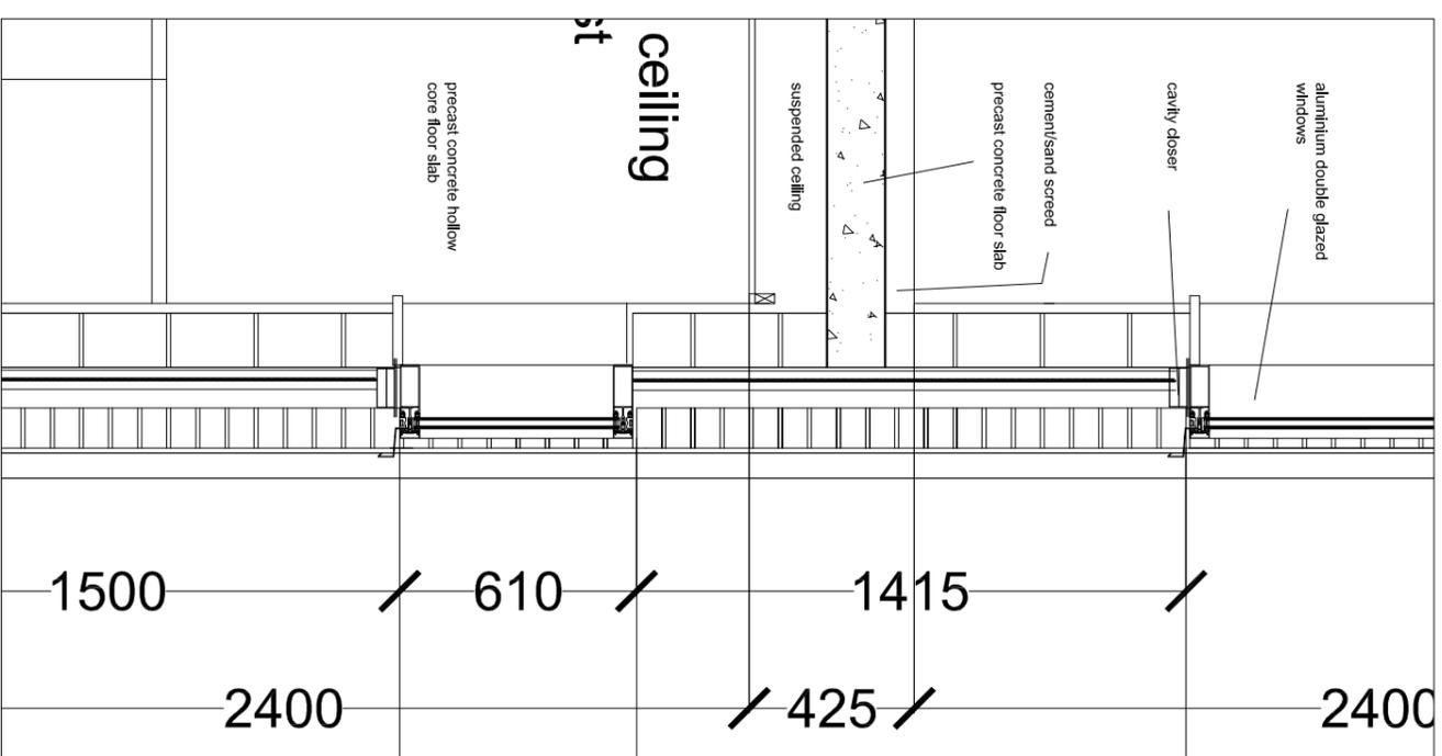
typical section through the external wall
